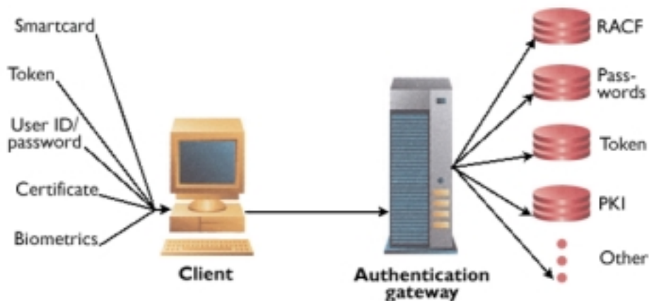
Figure 2. A secure single sign-on solution acting as an authentication gateway. All communications channels are encrypted.
